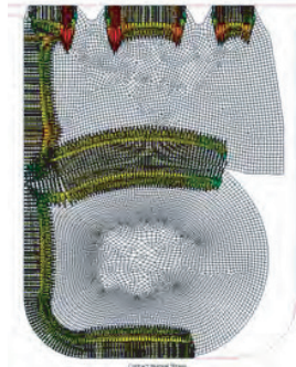
Contact Normal Stress at 300 bar
